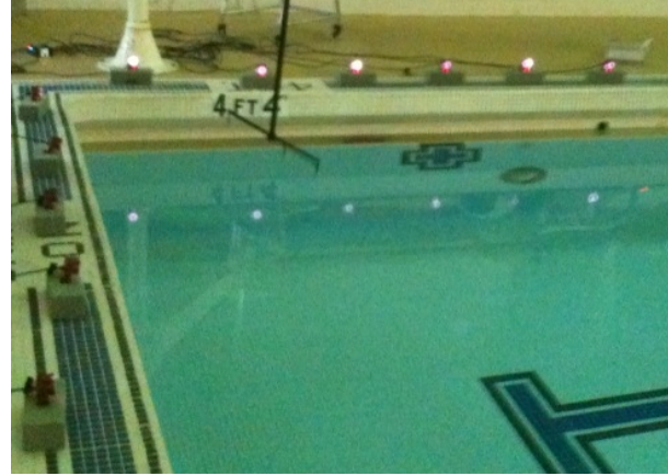
Figure 6. A ROBOTIC CART AND VARIABLE-CAMBER HYDROFOIL (LEFT) AND AN ARRAY OF CAMERAS ALONG TWO EDGES OF A POOL FOR OPTICAL MOTION TRACKING (RIGHT).
